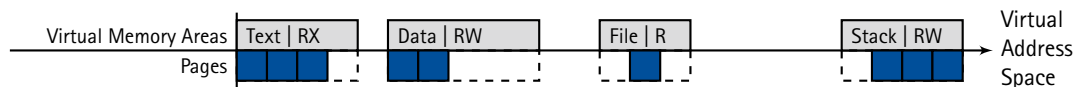
Figure 2.5 – A process address space defined through multiple virtual memory areas (VMAs): Each VMA has an individual set of flags and functions, e.g., access right (read, write, execute). Actual pages are typically mapped on demand.
